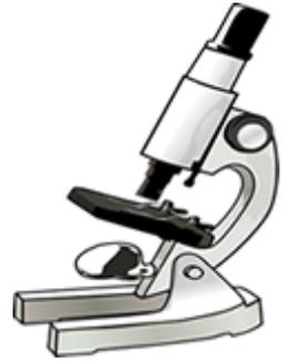
Light microscopes use either a bulb or a mirror (M) as their light source. Never use direct sunlight; it may damage your eyes. Color the light source yellow. The switch for this light is usually found on the base of the microscope, and sometimes on the power cord.
